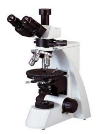
**XPL-2** series polarization microscopes are utilized polarize light to observe and research the matter which have double refraction features, the user can make single polarizing view, orthogonal polarizing view, cone light view. They are applied in geology, chemicals, physic and leechdom fields. They are also widely used to observe the crystal of liquid macromolecule polymer, biomedical polymer and liquid crystal.
